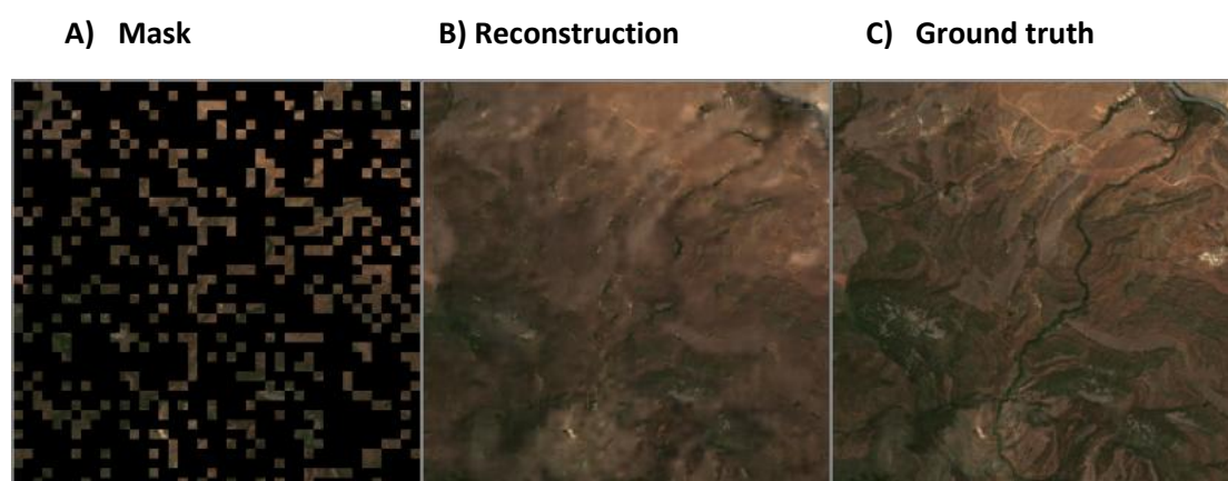
Figure 3-13: Example Sentinel-2 RGB image reconstruction (B) from a masked input image (A), compared to the ground truth (C).
